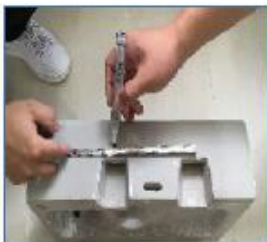
Measure the centre dimension between the slots on the basin
